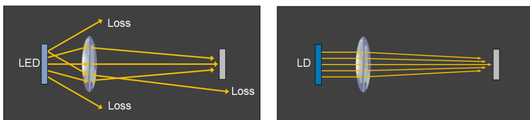
Figure 5: Collection of Light from an LED vs. a Laser Diode
