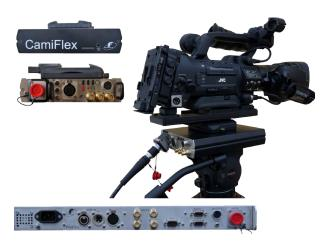
The fiber optic system can be used for the following JVC cameras: GY-HM170/200, GY-LS300, GY-HM600 Series and GY-HM800 Series. The headend can be used on a tripod or as a shoulder-mount version for the GY-HM8x0 series (and predecessors) via an adapter. You can transmit 1080P HD 3G signals, with a variety of control options (serial) and a 4-wire intercom link.
